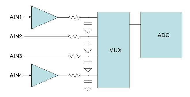
Figure 4. Amplifier(s) and Filter(s) Placed Before Multiplexer
