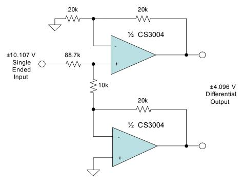
Figure 5. Single-ended-to-differential Conversion Circuit
