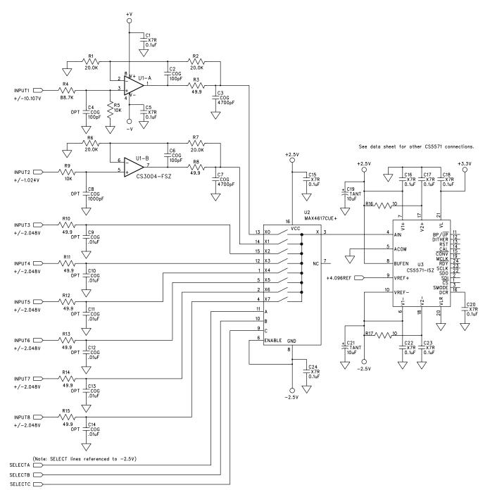
Figure 7. 8-input, Single-ended, Multiple Input Range, Multiplexed System
