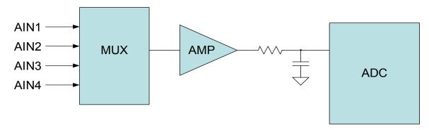
Figure 2. Amplifier and Filter between Multiplexer and ADC
