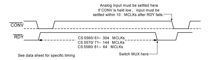
Figure 3. Multiplexer Timing Requirements
