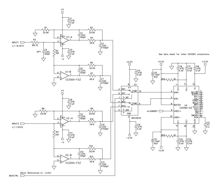
Figure 6. 2-input, Single-ended-to-differential, Multiple Input Range, Multiplexed System
